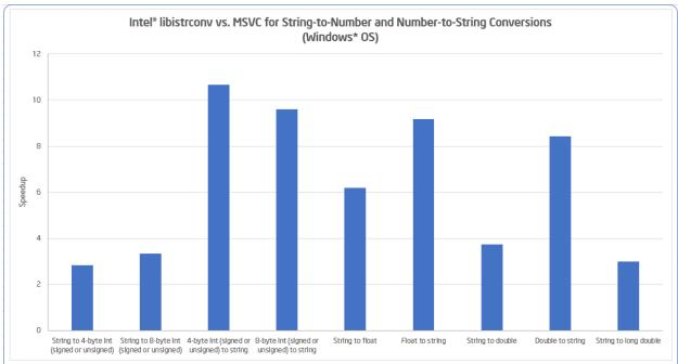
Configuration Info - Versions: Intel® C++ Compiler XE 2015 Beta, Microsoft\* C/C++ Optimizing Compiler Version 15.00.21022.08 for x64; Hardware: Intel® Core Processor i7-2700K, Quad-core CPU (8MB LLC, 3.5GHz), 8GB of RAM; Operating System: Windows Server 2008 R2 x64; Benchmark Source: Intel® Corporation. The reported speedup for each conversion is the geomean of measurements for different value ranges.
