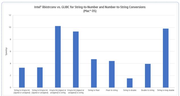
Configuration Info - Versions: Intel® C++ Compiler XE 2015 Beta, i686-apple-darwin11-llvm-gcc-4.2 (GCC) 4.2.1 (Based on Apple Inc. build 5658) (LLVM build 2336.11.00); Hardware: Intel® Core Processor i7-2635QM, Quad-Core CPU (6MB LLC, 2.0GHz), 8GB of RAM; Operating System: Mac\* OS X 10.0 (Darwin); Benchmark Source: Intel® Core proteins on the reported speedup for each conversion is the geomean of measurements for different value ranges.
